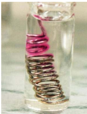
Immobilised urease producing ammonia from urea (indication by phenolphthalein)
